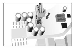
5. Connect extra cables from the cable pack to the sockets on the power supply only if needed. If you are going to plug the PCI-E cables into the PSU, they should go into the red sockets. If the red sockets are not being used for PCI-E, then they can be used for any other type of cable supplied in the pack that accompanies the PSU.
